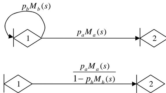
$$W_{1-2} = p_a M_a(s) [1 + p_b M_b(s) + (p_b M_b(s))^2 + \dots + (p_b M_b(s))^i + \dots] = \frac{p_a M_a(s)}{1 - p_b M_b(s)}$$
